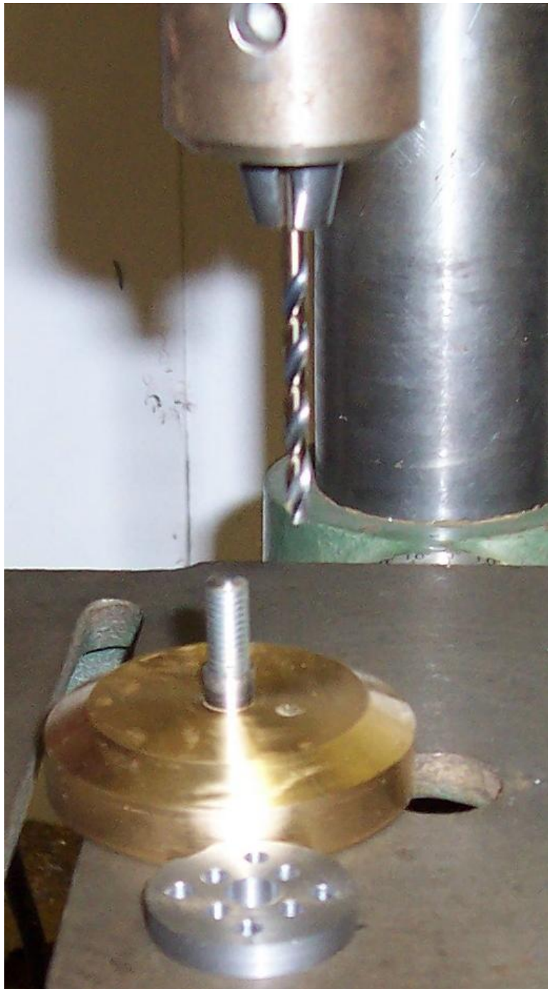
Figure 5 The 6mm nut has been turned down to leave a 7mm sleeve and spotting through the index plate. Please note that the index plate has an extra set of holes, these were later filled with iron wire
