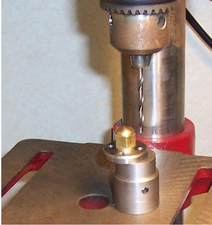
Figure 10 Drilling the 1/8" hole 5/16" deep for the locating peg
