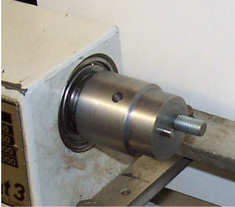
Figure 12 The tool screwed to the lathe
