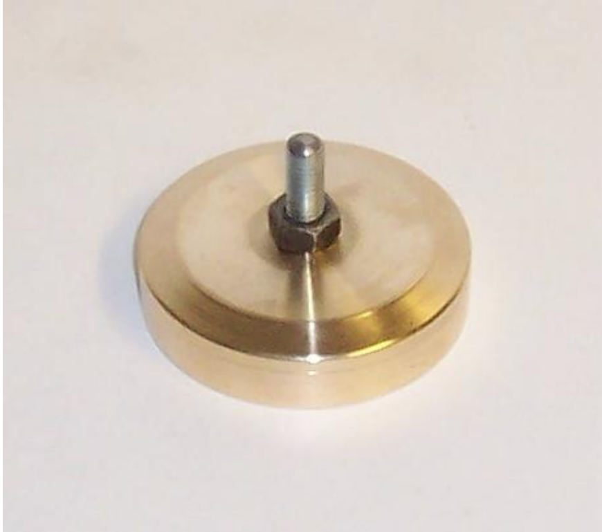
Figure 2 6mm Studding secured with Loctite and a 6mm nut
