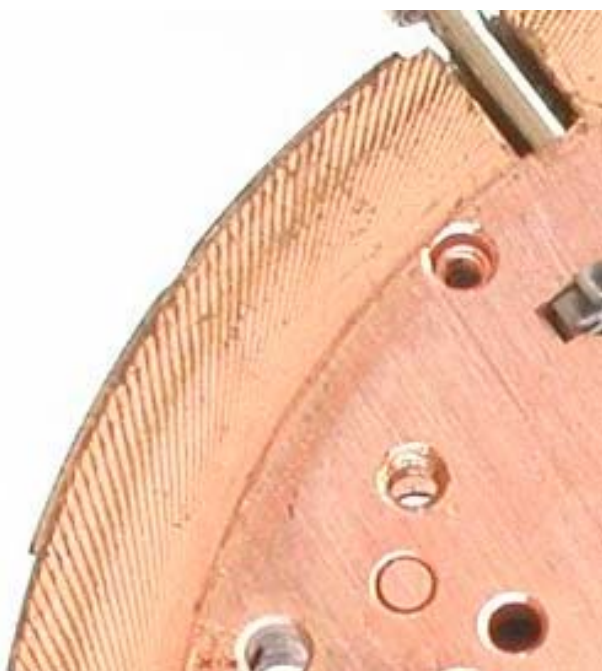
Close-up of 'Arabesque' finish on parts of the plate rim creating a strobe-like effect under certain light conditions
