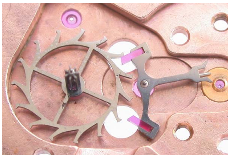
Calibre 551 escape wheel and pallet lever showing the jewelled entry and exit pallets
