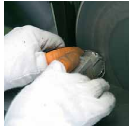
Only a handful of craftsmen still have the requisite skills to use the Zaratsu method of polishing, which enables them to produce results that cannot be achieved in any other way. It is used on the finest Grand Seiko watches.
