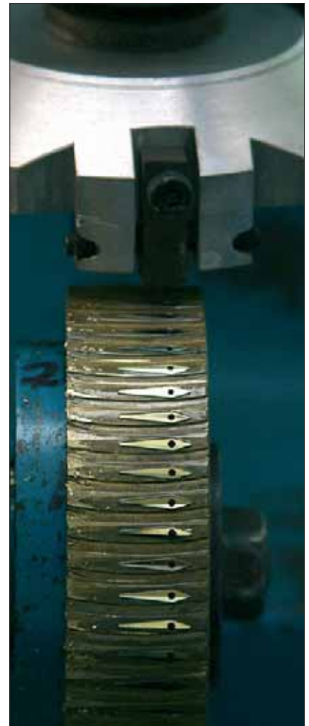
This diamond cutting tool applies a superb finish to watch hands, but relatively few can be polished at once.
