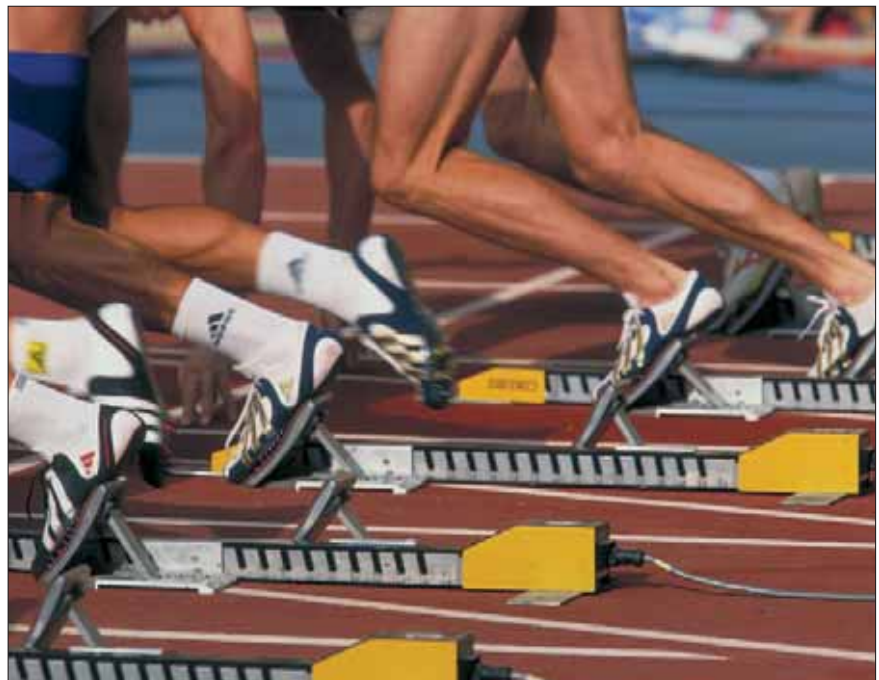
These pressure-sensitive starting blocks, introduced in 1995, gave officials new data to detect false starts.
