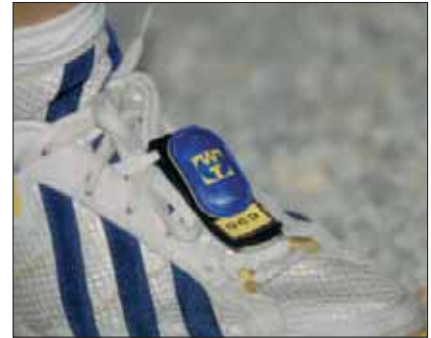
The latest transponder technology is now used to give instant times and positions in marathons, cross-country and ski races.
