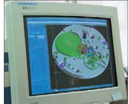
Although the 9S55 is finished to the highest traditional standards, it was designed using the latest 3D Computer Aided Design (CAD) software. It can be viewed on-screen from any angle and the software can simulate the movement in operation.
