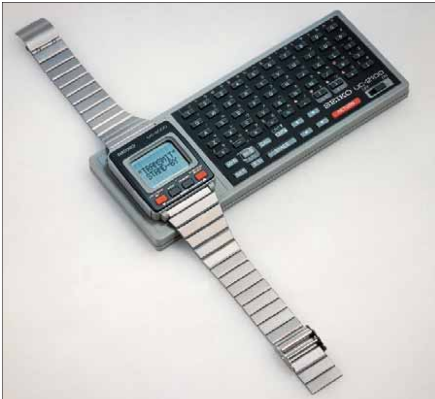
The wrist computer, launched in 1984, was in two parts, the wrist mounted portion and the controller. It represents a very complex marriage of quartz, LCD and IC technologies, the fields in which Seiko has played a leading role.
