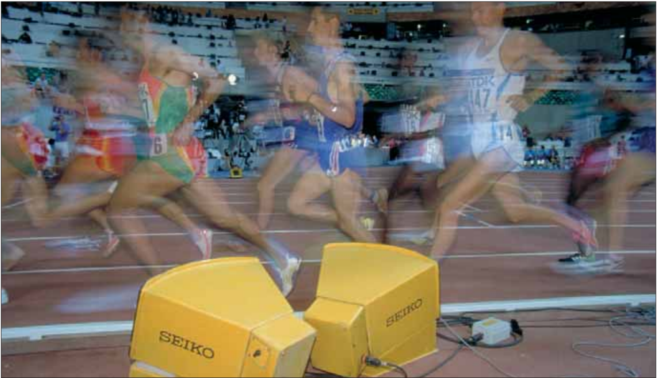
Loudspeakers convey the starter's signal to each lane individually, to counteract the delay of sound travelling through the air.
