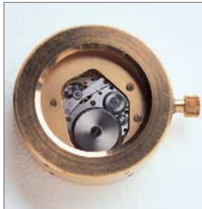
By 1968, Seiko was experimenting with even faster movements. The barrel housing the mainspring was increased in size to accommodate the stronger mainspring and the movement shape was changed to a “deformed pentagon”. This was Seiko’s ultimate competition movement.
