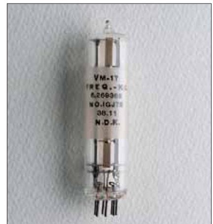
The quartz crystal oscillator in the QC-951 was housed in a large vacuum tube 10cms long. It had a frequency of 6,269.388Hz and its circuitry included eleven germanium transistors and three silicon diodes.
