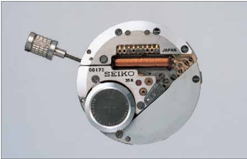
The Astron movement began the quartz revolution. The screws suggest that it could be dismantled simply, but when it was first introduced no watch repairer outside Seiko would have known what to do with it.
