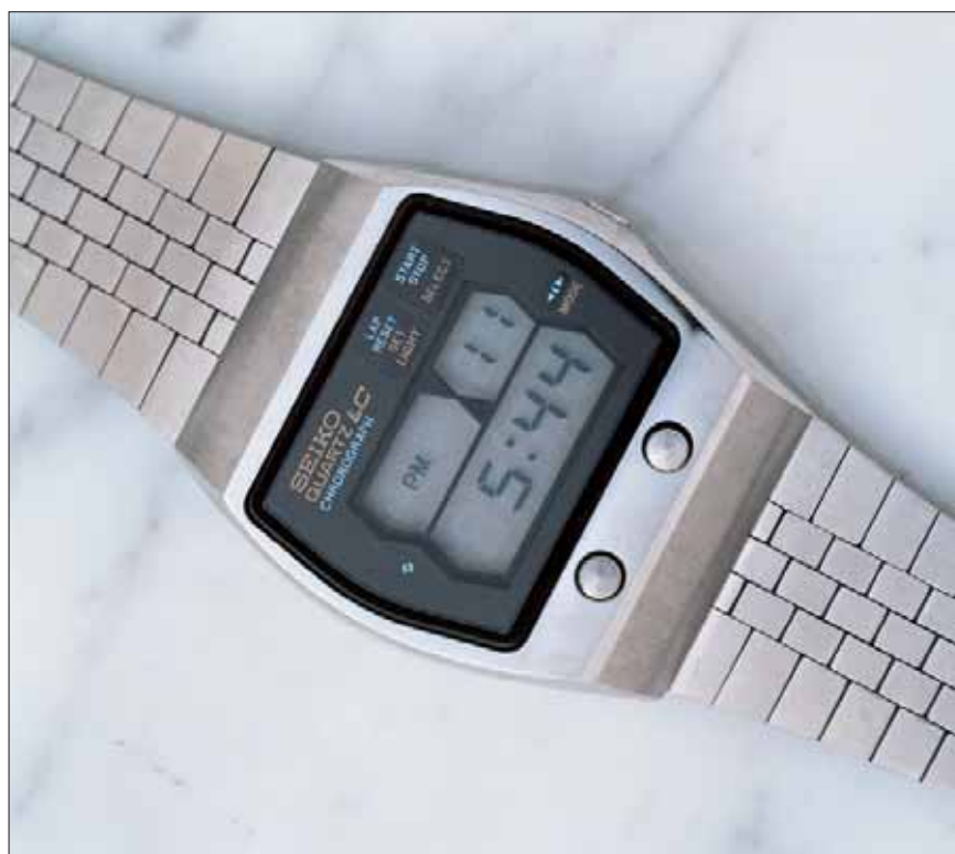
In 1975 Seiko launched the world's first digital quartz watch with a chronograph, the 0634. It could record time to 1/10 of a second and had a lap time function. It also incorporated an internal light, so that it could be seen clearly in the dark.
