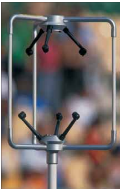
Ultrasonic wind gauges measure the wind speed. A reading of more than two metres a second invalidates a world track record.
