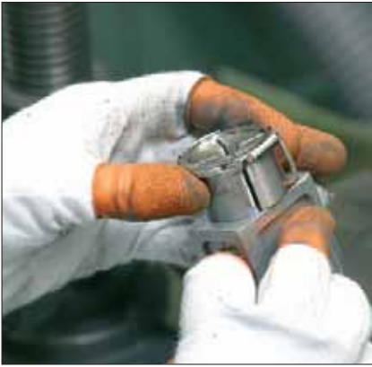
A case is examined after it has been polished using the artistic Japanese Zaratsu technique.
