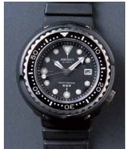
The Professional 600M had a titanium case and was water resistant to 600m. It overcame the problems associated with helium gas during prolonged saturation dives and met the needs of professional divers. It was an enormous improvement over earlier models. At first, it was fitted with an automatic hi-beat movement, but later a quartz movement was used.
