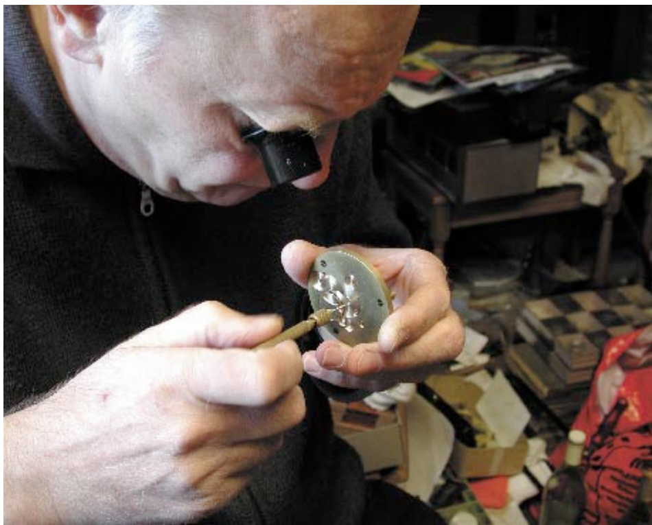
Top: Several tourbillons in various stages of completion are typical treasures found lying about Miklosch's workshop. Bottom: Broaching holes to final size.
