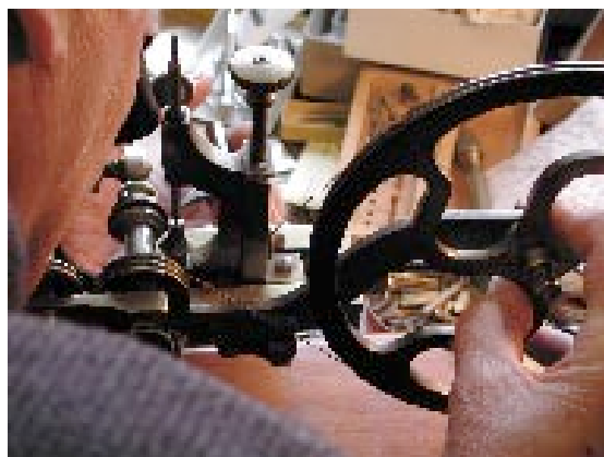
Top: The “hi-tech” work of Miklosch. He uses an 8mm watchmaker’s lathe to cut wheels for his watches.
