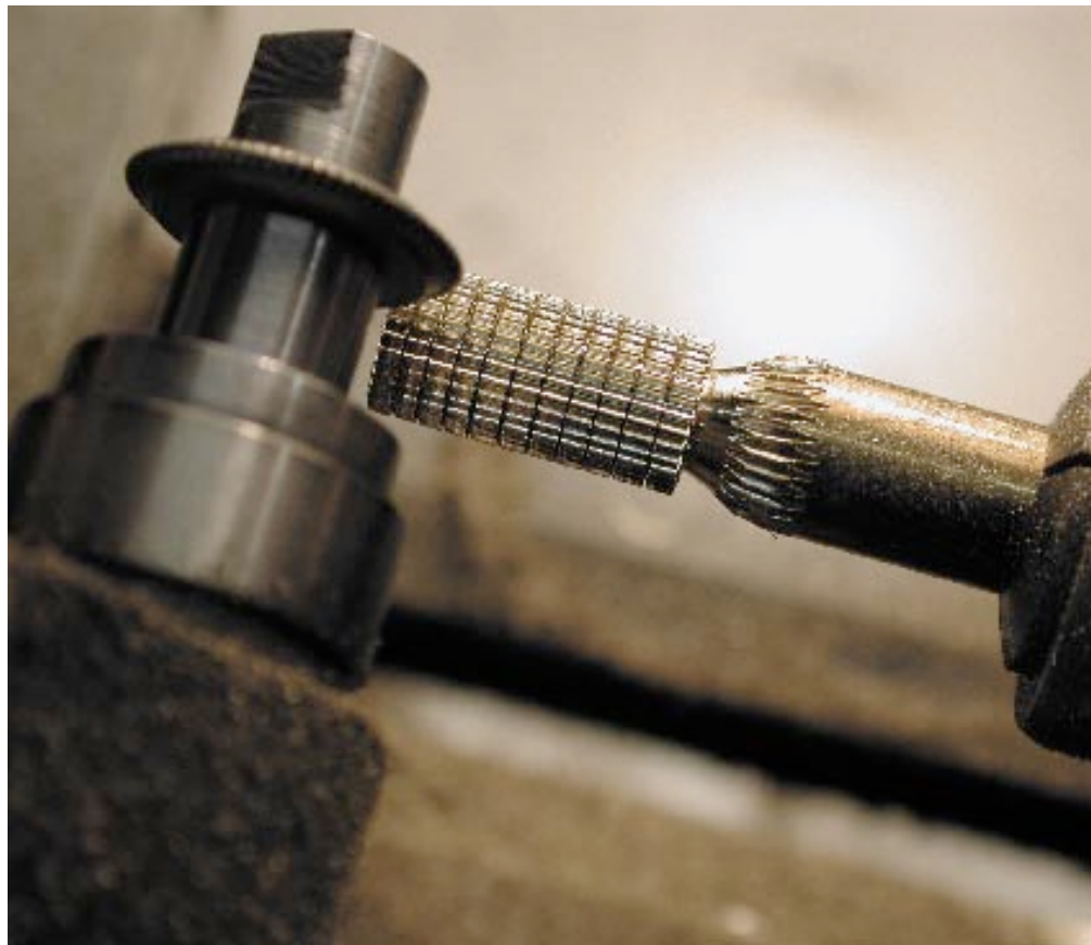
Top: The “hi-tech” work of Miklosch. He uses an 8mm watchmaker’s lathe to cut wheels for his watches.
