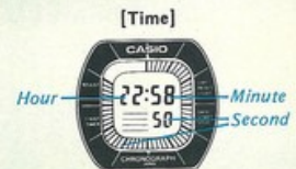
Continuous digital display of hour, minute and second in 24-hour format. Seconds are also shown in analog display.
