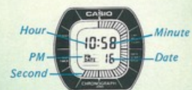
Continuous digital display of hour, minute, am/pm and date. Seconds are shown in analog display.
