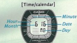
Continuous digital display of month, date and day. Hours are shown by a dot indicator. Minutes are shown in analog display.
