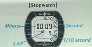
Measures net/lap/1st-2nd place times with accuracy of 1/10th second up to one hour.
