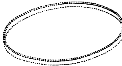
A—GASKET, Bezel—Material No. 703 Shape of gasket before it has been installed on bezel in circular as shown here in phantom view.
