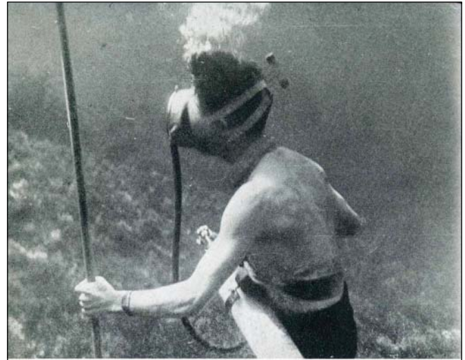
The ancestor of our aqualung diving apparatus was Le Prieur's 1933 compressed-air cylinder.
