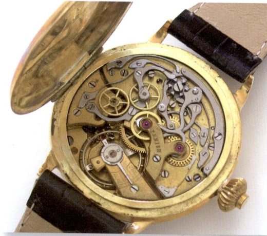
Single pusher chronograph about 1920, manual winding, 18 K gold case, case diameter 40 mm, nickel- and gold-plated movement, operating star, caliber Raymond (?), enamelled face, spiral shaped tachymeter starting at 20 km/h, 30 minutes' counter, chronograph pusher in the crown. (Zenith collection)
