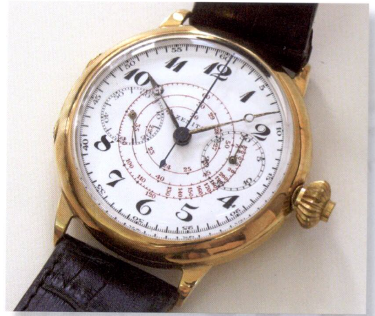
Single pusher chronograph about 1920, manual winding, 18 K gold case, case diameter 40 mm, nickel- and gold-plated movement, operating star, caliber Raymond (?), enamelled face, spiral shaped tachymeter starting at 20 km/h, 30 minutes' counter, chronograph pusher in the crown. (Zenith collection)
