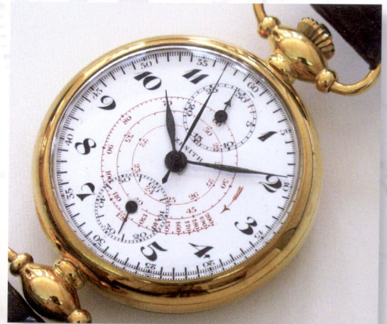
Single pusher wrist chronograph, about 1920, manual winding, 18 K gold case, case diameter 39 mm, case serial number 61803, Caliber Raymond (Valjoux GH, 15''), nickel-plated movement, operating star, crown at 12 (three functions by pressing the crown), enamelled face, red spiral shaped tachymeter 20-200 km/h, bow shaped moving lugs, hinged case. (Zenith collection)
