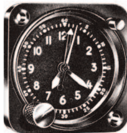
Former cockpit clock, below left. The vertical crown is used to set the second time.
