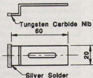
Fig 5. Brass Holder for Nib Blank
