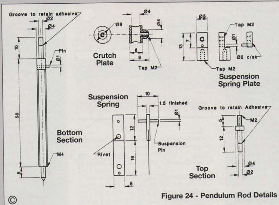
Figure 24 - Pendulum Rod Details
