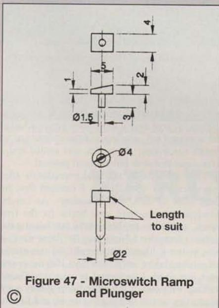
Figure 47 - Microswitch Ramp and Plunger
