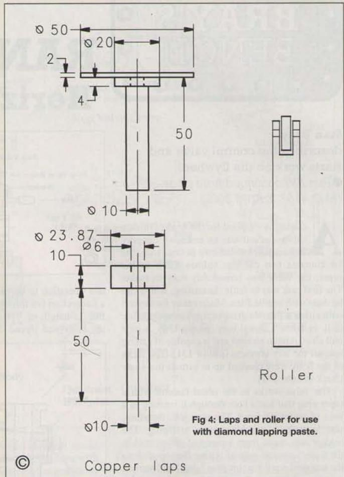
Fig 4: Laps and roller for use with diamond lapping paste.
