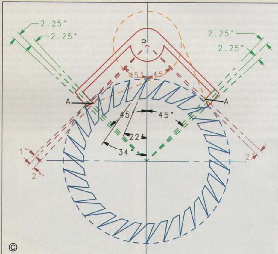
Fig 2: To construct the escapement
