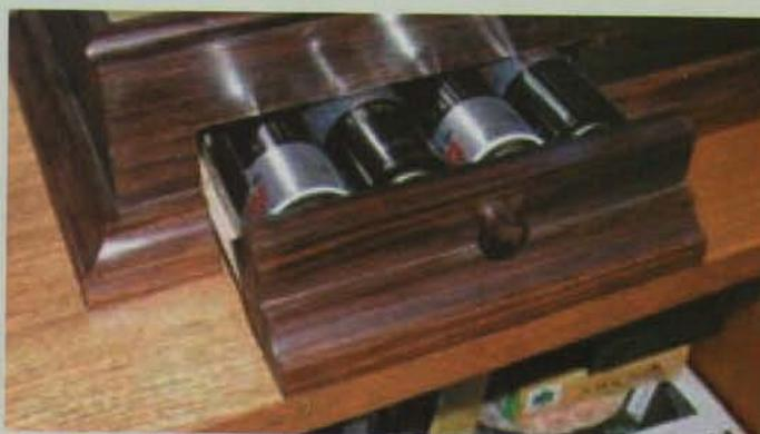
A drawer to the front houses the dry cells which supply power to the Archimedes screw drive motor.
