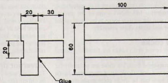
Fig 6. Perspex Guide for Brass Holder
