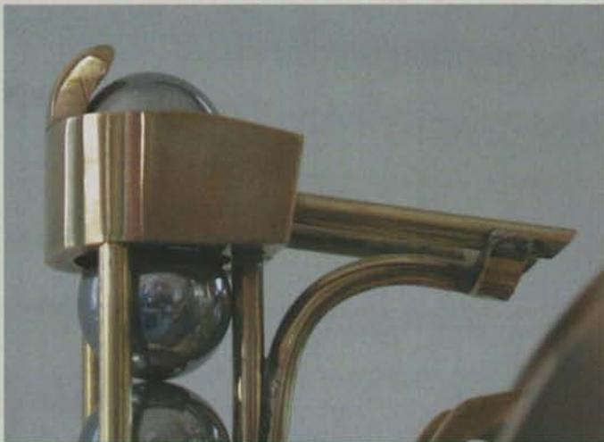
The deflector block, which requires care in its manufacture, is positioned at the top of the vertical track and delivers the balls to the Ferris wheel.
