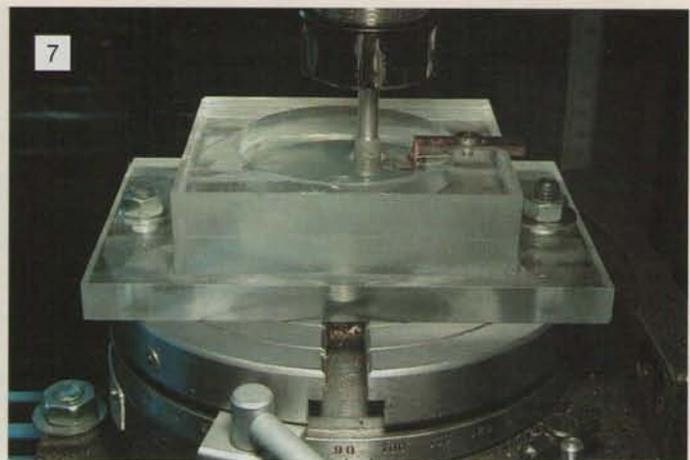
Method 2 for finishing the pallet nibs using a milling machine and rotary table. Note the Perspex bath to contain the cutting fluid.
