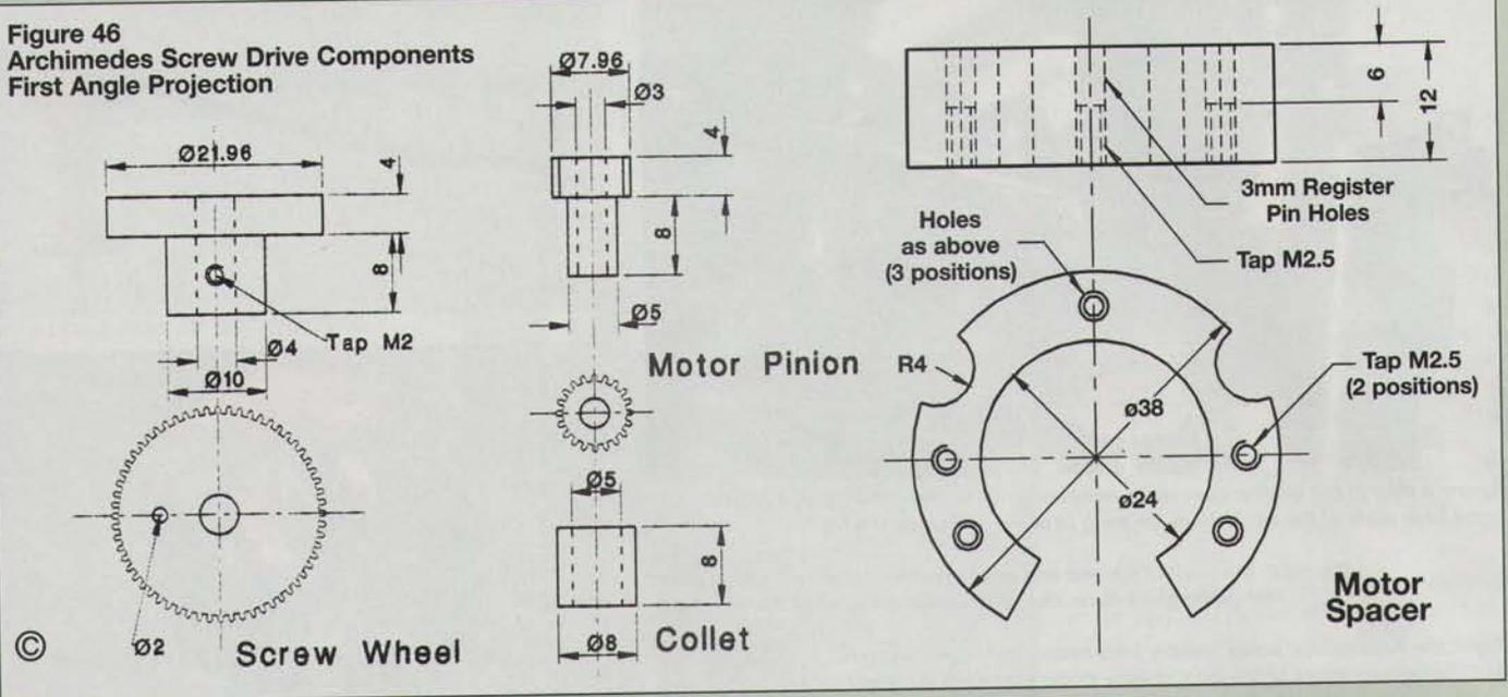
The replacement has a different output speed, which can be accommodated by modifying the gear ratio between the motor and the Archimedes screw. The design is flexible so there is no reason why another type of motor could not be used. It is simply a case of the appropriate modifications being made for mounting the motor. Readers who have come this far with the clock should have no difficulty sorting out the necessary details.
