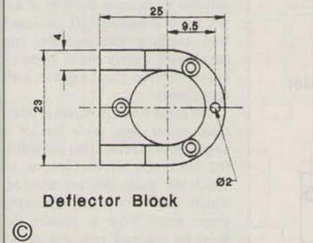
the block to 25 x 23 x 14mm. Mark the centre line and drill and ream a 15mm dia. hole, 11.5mm from the 22mm edge. Set the radius of the boring head to 7.5mm. Grip the block in a vice on the milling machine inclined at an angle of 10deg. off the vertical and bore the semicircular recess that forms the start of the delivery track.
