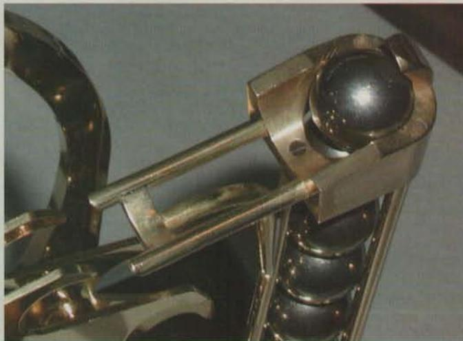
This view of the deflector block and track reveals its construction. The ball is about to run out onto the Ferris wheel.
