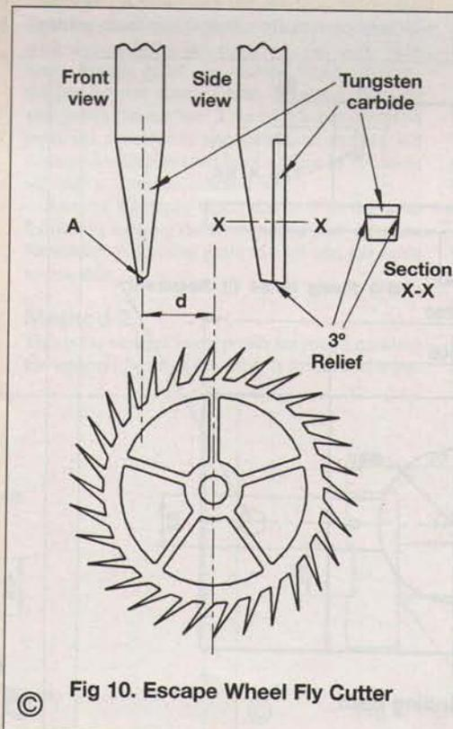
**Fig 10. Escape Wheel Fly Cutter**
