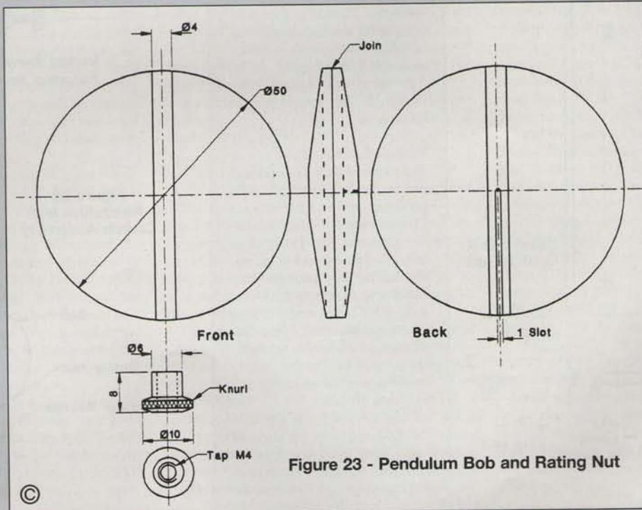
Figure 23 - Pendulum Bob and Rating Nut
