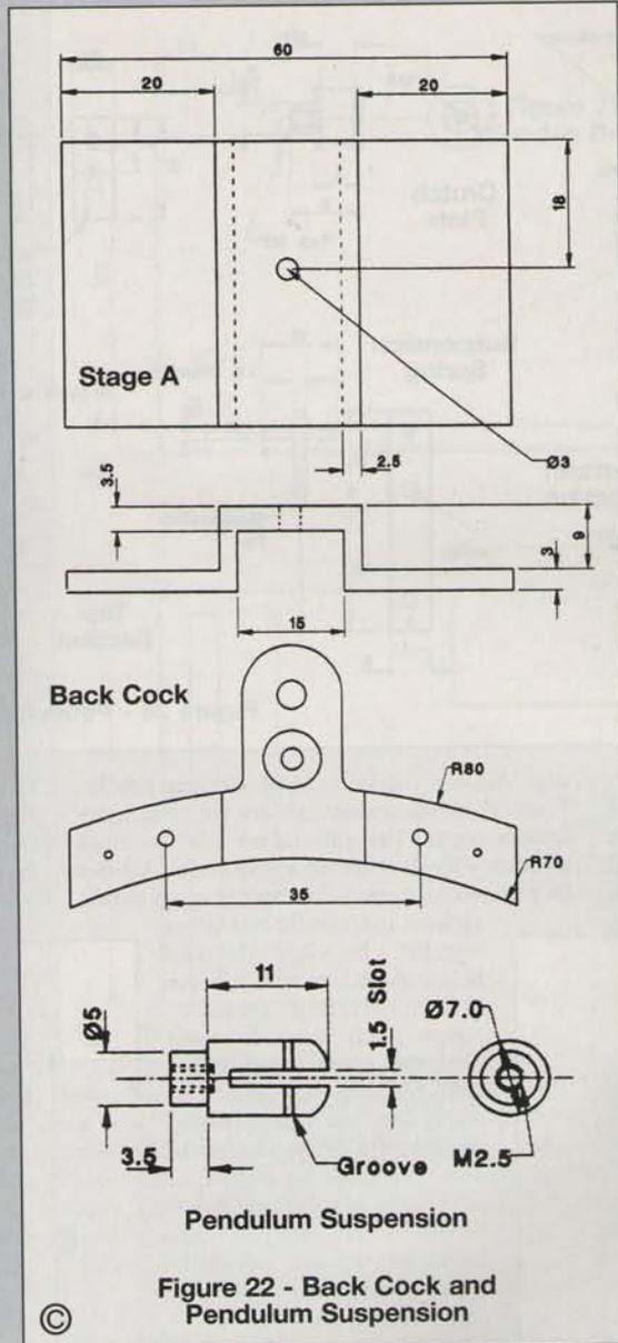
Figure 22 - Back Cock and Pendulum Suspension
