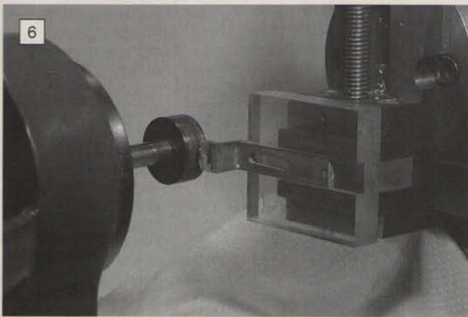
Method 1 for finishing the internal faces of the pallet nibs using a vertical slide and a lap mounted in the lathe headstock spindle.
