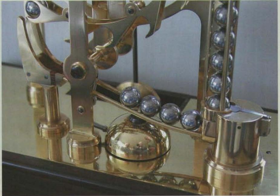
The contacts and entrance track assembly with four balls waiting to enter the guide. The insulation material between the contacts is clearly visible.
