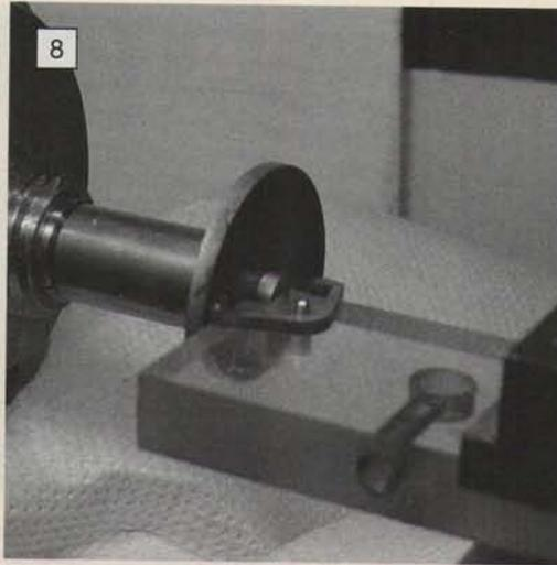
**Lapping the outside curved faces of the pallet nibs using a face lap mounted in the lathe spindle. Note the paper towels to protect the lathe bed.**
