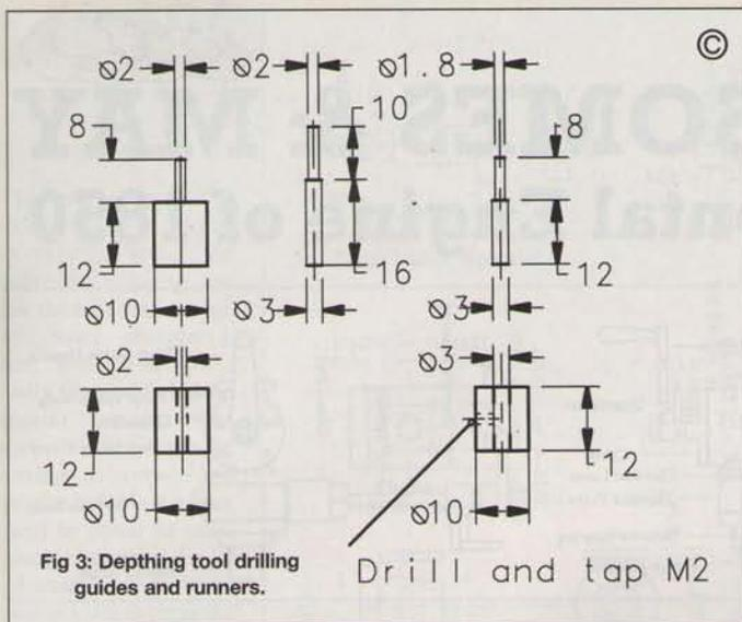
Fig 3: Depthing tool drilling guides and runners.
