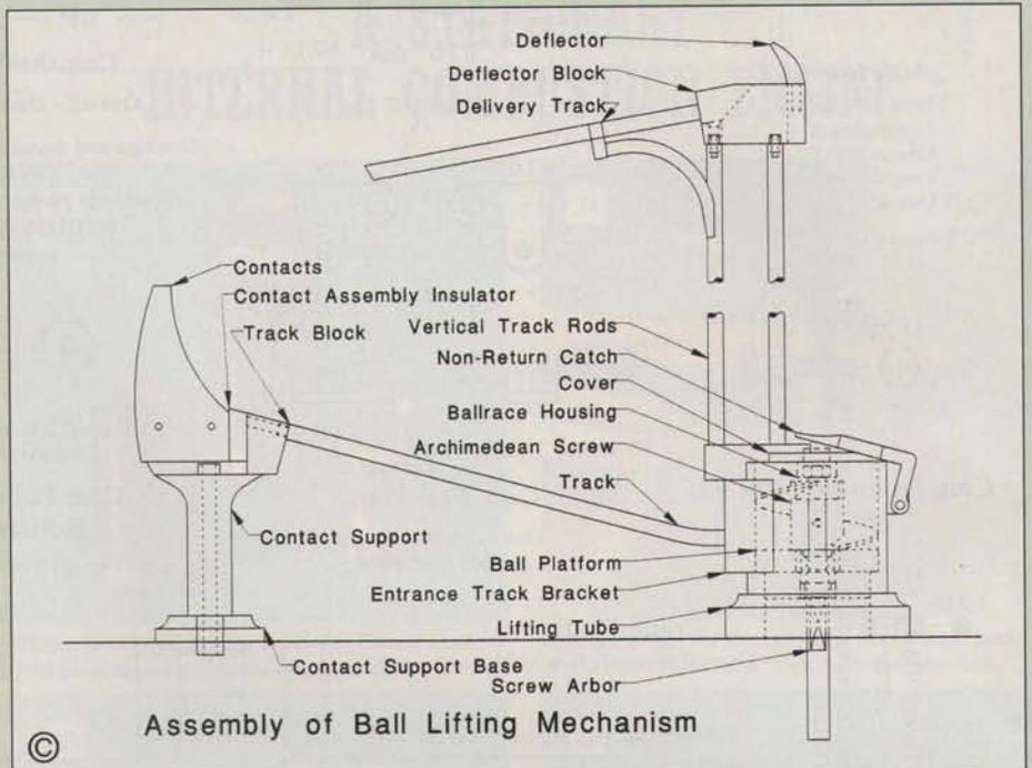
screw must be just below the surface of the shaft or it will foul the balls as the shaft turns.
