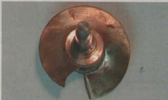
Right: the Archimedes' screw looking from below. The edge chamfers and the hooked shape of the leading edge of the screw are apparent.
