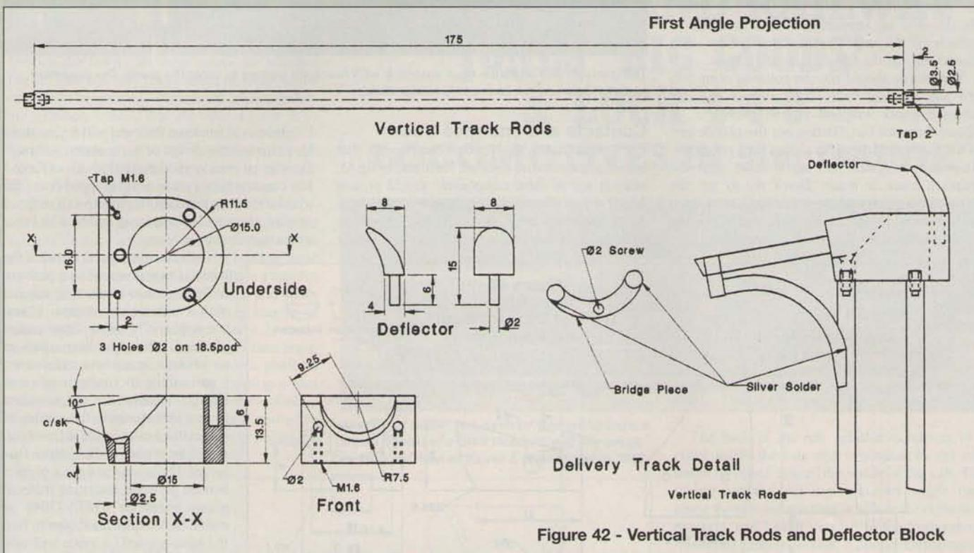
Figure 42 - Vertical Track Rods and Deflector Block
