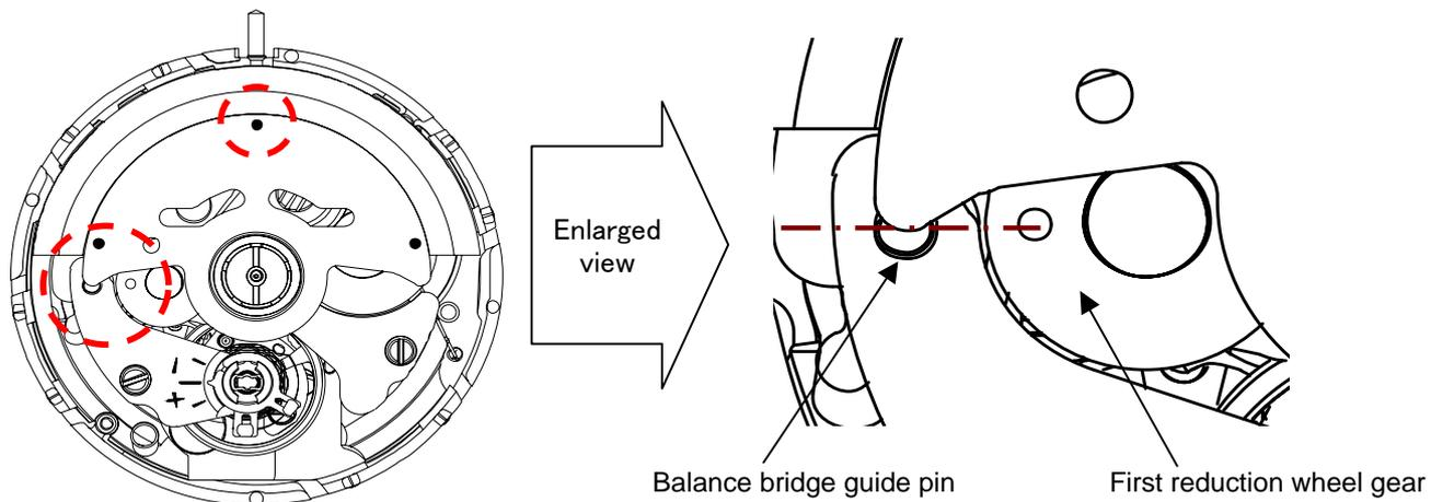
**2.Disassembling / assembling of the First reduction wheel**
