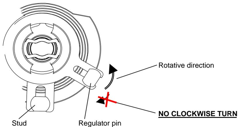
**5.Second reduction wheel and pinion screw**
