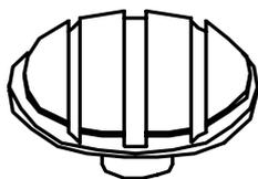
⑰ Second reduction wheel and pinion screw
